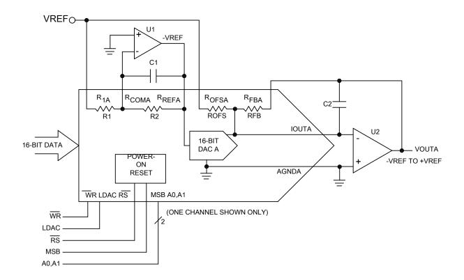
FIGURE 7. 16-bit 4-quadrant multiplying DAC with minimum of external components.
